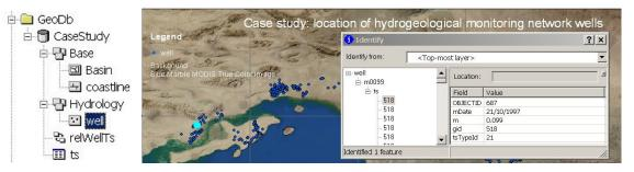
Fig. 23 – Snapshot of an ESRI geodatabase skeleton in ArcCatalog and of an editing session in ArcMap accessing data through a relationship class
