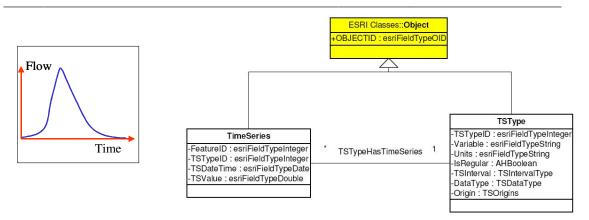
CRWR, 2010 Fig. 16 - Hydro data model: key tables schematic architecture
