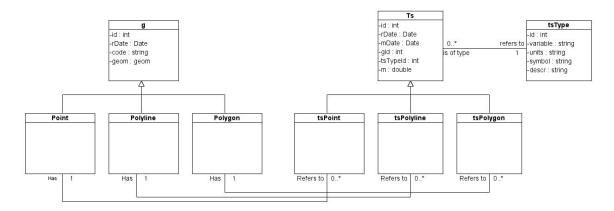
Fig. 20 - UML data model for spatio-temporal data management: PostGIS design based on table inheritance
