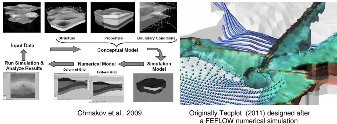
Fig. 6 - Information flow in building complex groundwater numerical models and advanced visualisation of 3D density-dependent flow near a coastline
